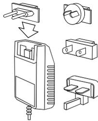
② Connect the battery charger cable to the lower end of the telephone (the arrow printed on the connector must **not** be visible when the plug is inserted) and the other end into a power supply socket (100V – 240V).
