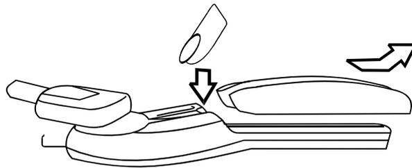
② To insert the SIM card, use the relevant guides ensuring that the bevelled edge of the SIM card is facing the upper part of the telephone and that the gilded contacts are facing the telephone (and thus not visible).
