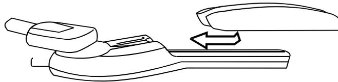
**NOTE:** For correct recharging the ambient temperature (**not** that on the display) must be between 0° and +45° C.
